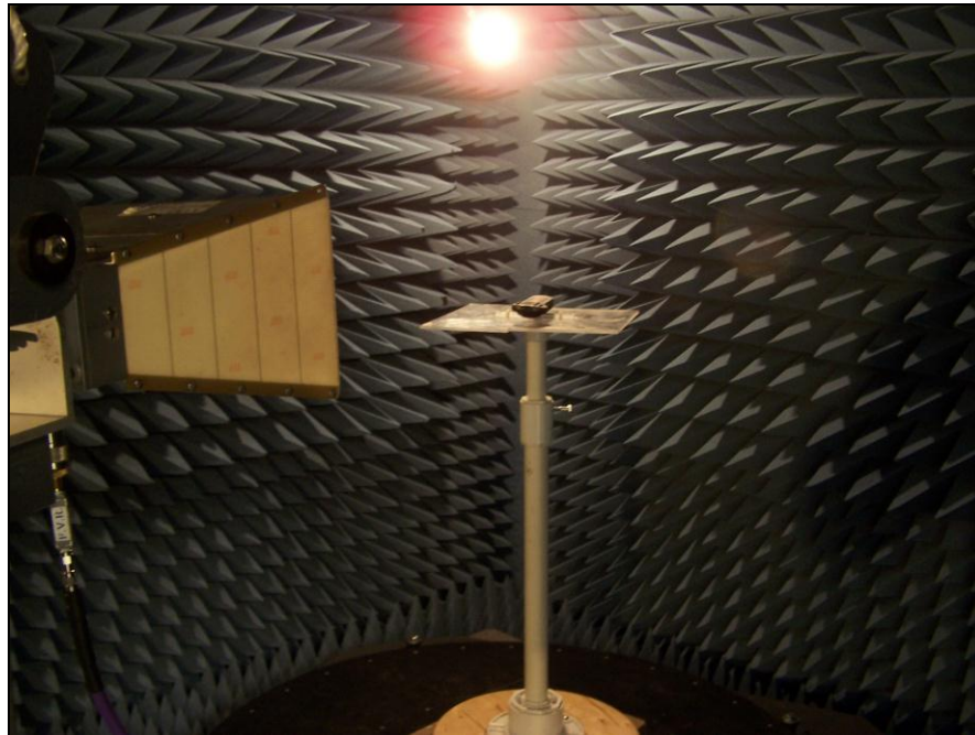
Photograph 4. Radiated Spurious Emissions, Test Setup
