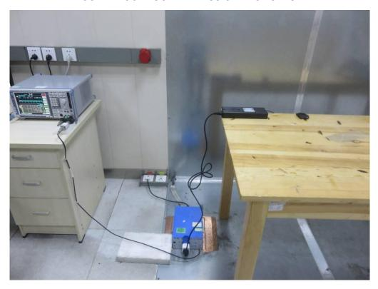
FCC RADIATED EMISSION TEST SETUP
