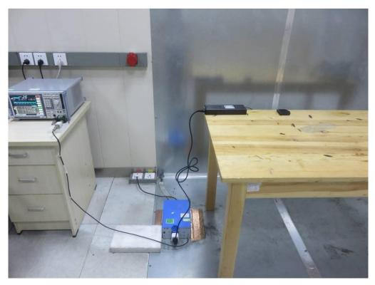
FCC RADIATED EMISSION TEST SETUP
