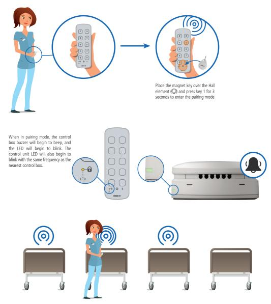
In pairing mode, the light/sound frequency will increase when the HB200 gets closer to a control box.
