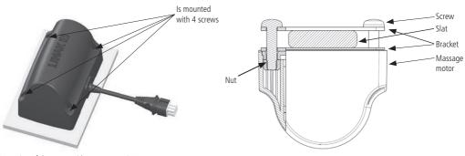
Mounting of the screw with max. torque 2 Nm
