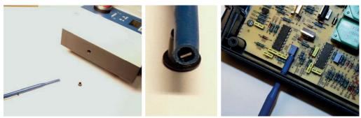
Only the end with the lowered notch must be used for adjustment of the potentiometer.
