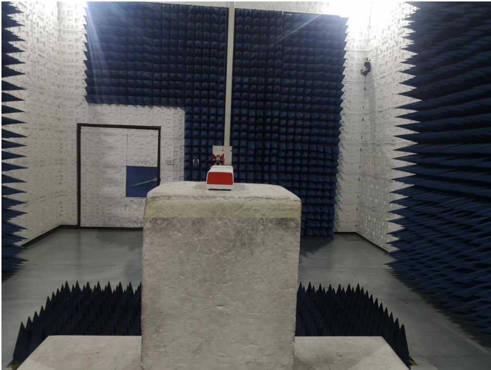
RADIATED EMISSION TEST SETUP ABOVE 1GHZ
