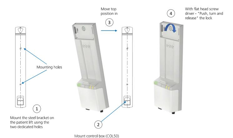
\* The bracket kit includes 3 M5x10 mm screws. This is a special screw type (Bossard Ecosyn-grip) with a wide collar for improved fixing. Screw torque for the screw betweeen COL50 and the bracket must be max. 1 Nm.
