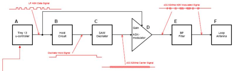
The calibrated internal RC Oscillator provides a 4.8 MHz clock.
