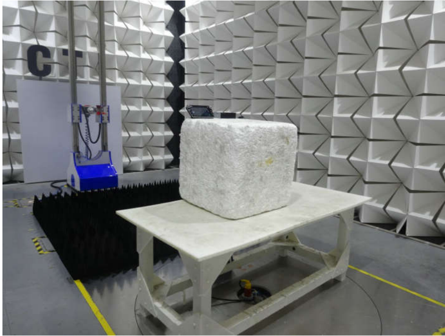
Radiated spurious emission Test Setup-3(Above 1GHz)
