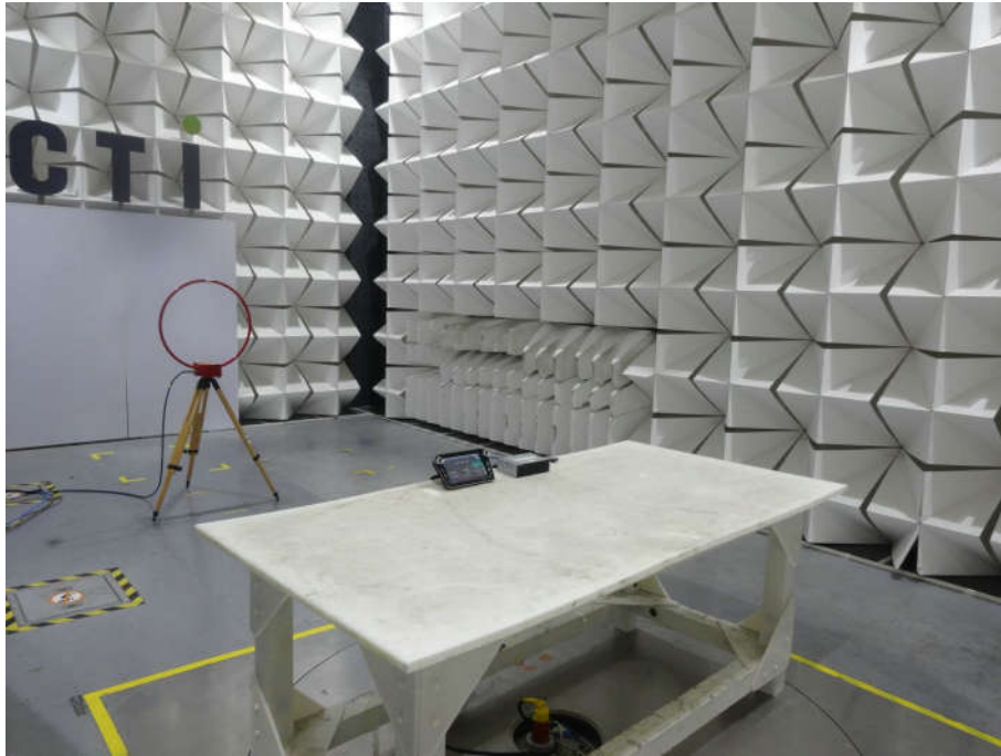
Radiated spurious emission Test Setup-1( 9K-30M )
