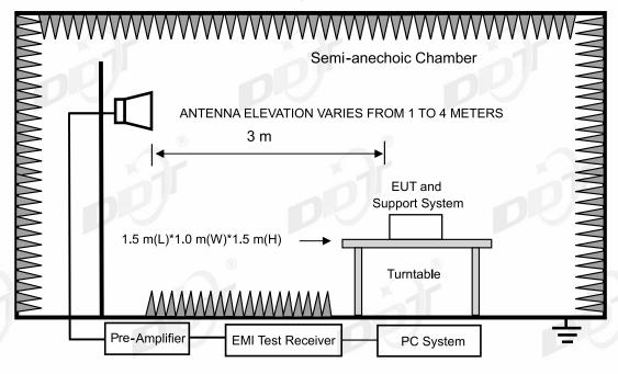
Note: Install an appropriate filter at the input of the measurement system power amplifier. This filter can attenuate the fundamental emission of the EUT and allow an accurate measurement of the associated harmonics and spurious emissions. The filter had been characterized, and the attenuation loss factors had been accounted for in the measurement results.
