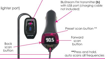
BluStream FM module with control button and built-in mic (a) and hidden cable management
