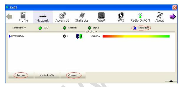
You can click the button *Rescan* to find which AP is in range, they will show on the window. Choice one you want to connect, and click the button *connect* to finish the connection. An infrastructure connection is completed.
