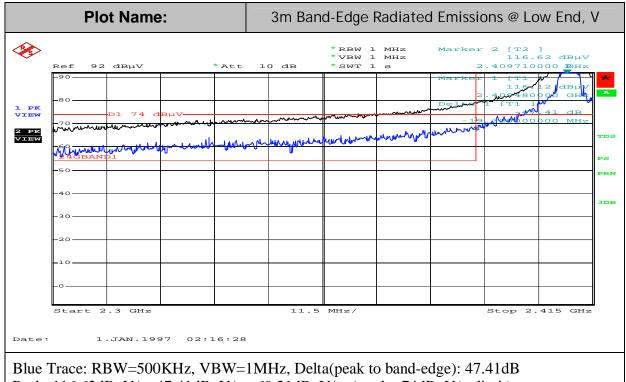
Peak: 116.62dBuV/m-47.41dBuV/m=69.21dBuV/m ( under 74dBuV/m limit)
