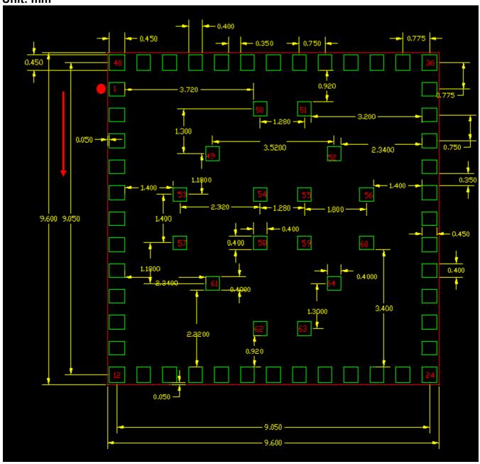
Note: AzurWave will provide AW-GH381 Top View FootPrint DXF file for customer reference.
