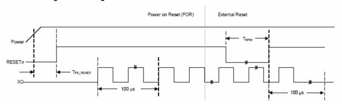
Note: Pin 39 RESETn is not needed for proper operation due to internal power-on reset logic.
