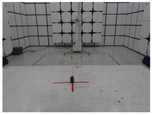
RADIATED EMISSION TEST SETUP ABOVE 1GHz
