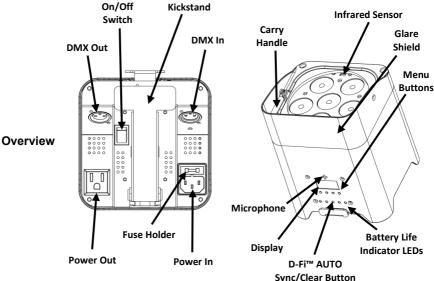
AC Power This product has an auto-ranging power supply that can work with an input voltage range of 100~240 VAC, 50/60 Hz.
