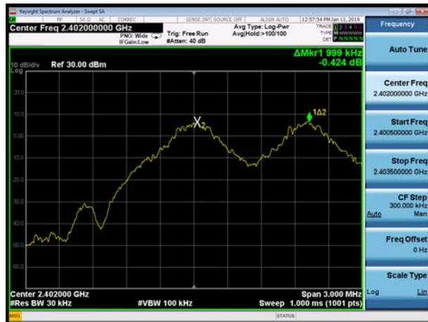
BT DH5 CH39, Carrier frequency (MHz): 2441
