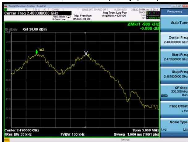
BT DH5 CH78, Carrier frequency (MHz): 2480
