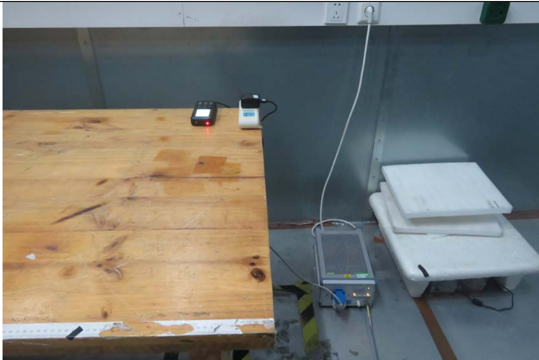
Picture 3 Conducted Emission Test Setup
