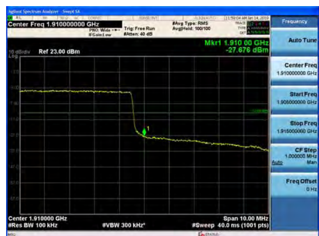
LTE Band 2 10MHz QPSK 100%RB CH-High
