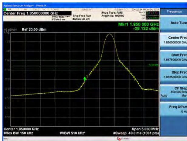
LTE Band 25 15MHz QPSK 100%RB CH-Low
