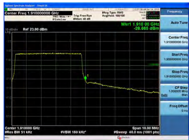
LTE Band 2 10MHz 16QAM 1RB CH-High
