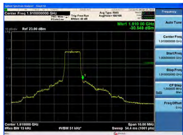
LTE Band 2 1.4MHz QPSK 100%RB CH-High
