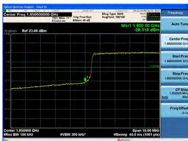
LTE Band 25 10MHz QPSK 100%RB CH-Low
