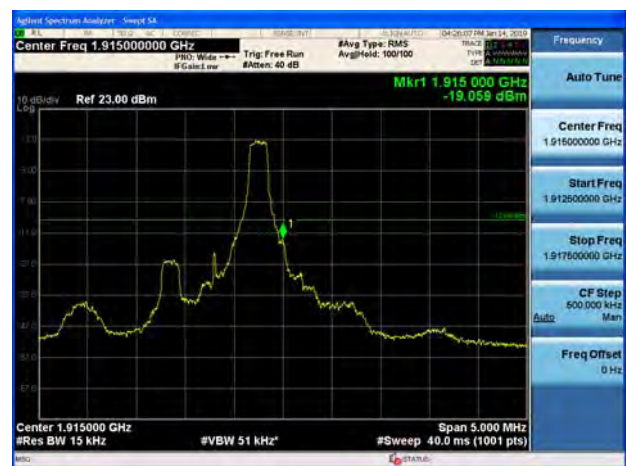
LTE Band 25 1.4MHz QPSK 100%RB CH-High
