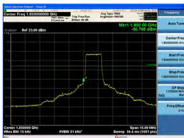
LTE Band 25 1.4MHz QPSK 100%RB CH-Low
