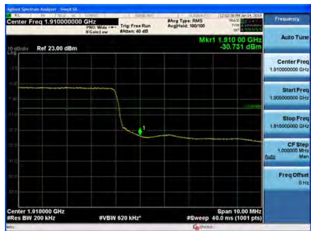
LTE Band 2 1.4MHz 16QAM 1RB CH-High
