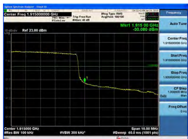
LTE Band 25 10MHz QPSK 100%RB CH-High
