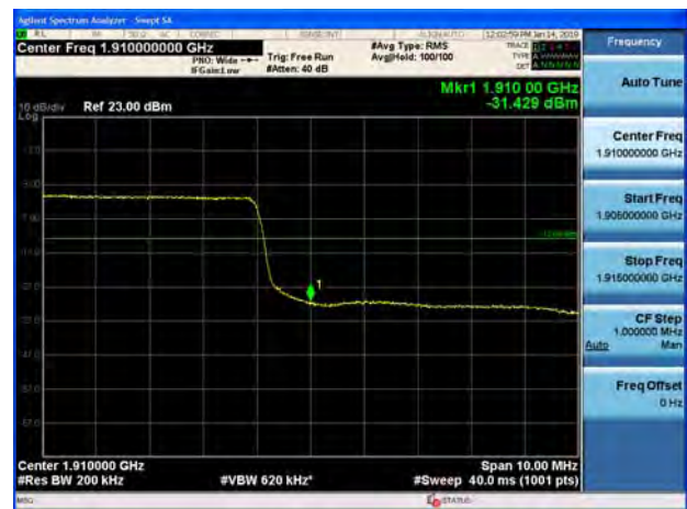
LTE Band 25 1.4MHz QPSK 1RB CH-High
