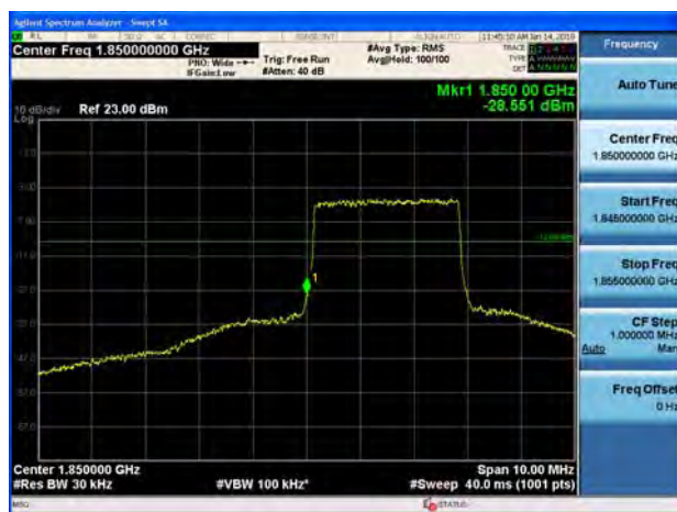
LTE Band 2 5MHz 16QAM 1RB CH-Low
