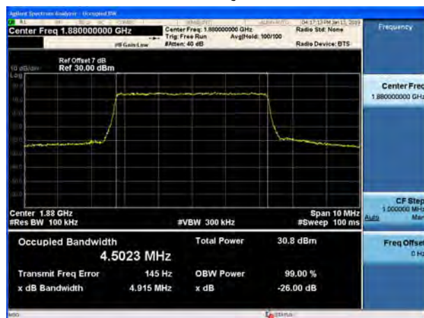
LTE Band 2 5MHz QPSK CH-High
