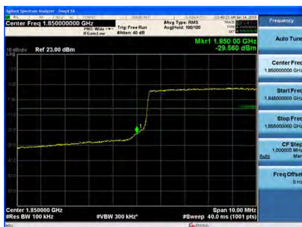
LTE Band 2 10MHz QPSK 100%RB CH-Low
