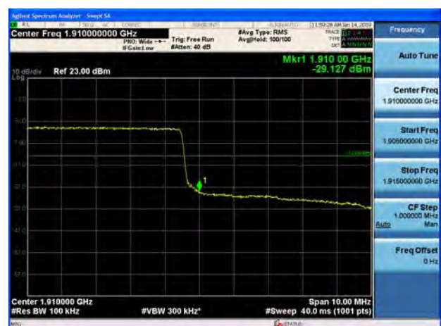
LTE Band 2 10MHz 16QAM 100%RB CH-High
