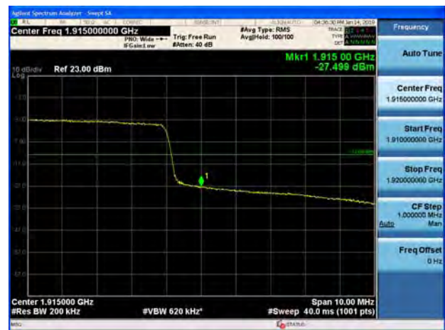
LTE Band 25 1.4MHz 16QAM 1RB CH-High
