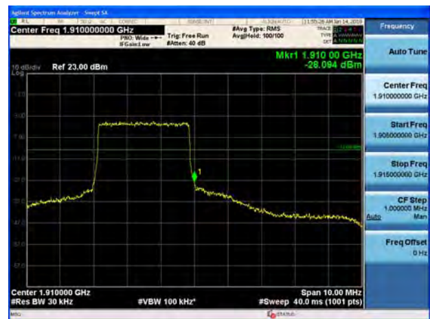
LTE Band 2 5MHz QPSK 1RB CH-High
