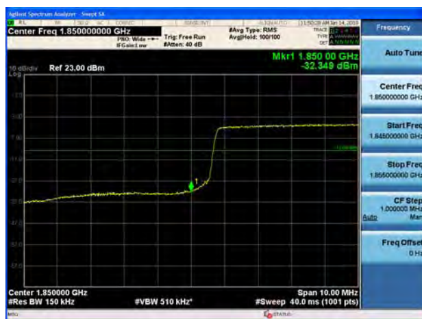
LTE Band 2 20MHz 16QAM 1RB CH-Low
