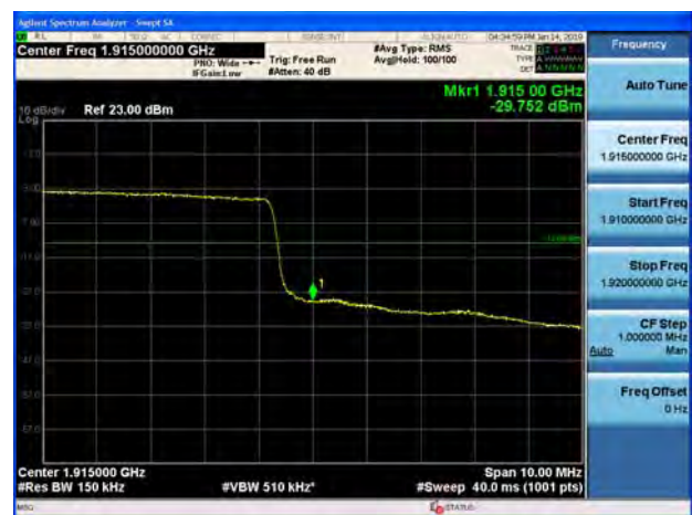
LTE Band 25 20MHz 16QAM 1RB CH-High
