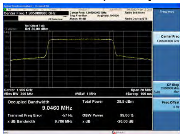
LTE Band 2 10MHz QPSK CH-High
