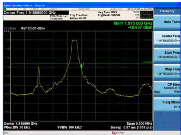
LTE Band 25 3MHz QPSK 100%RB CH-High
