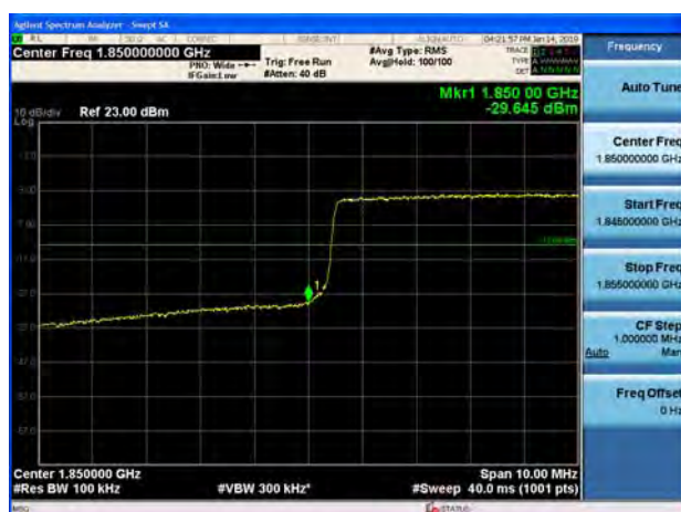
LTE Band 25 10MHz 16QAM 100%RB CH-Low
