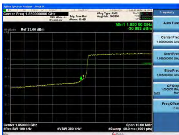
LTE Band 2 10MHz 16QAM 100%RB CH-Low
