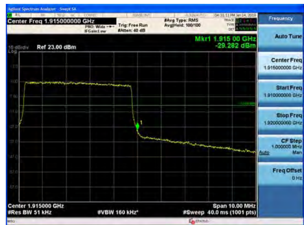
LTE Band 25 10MHz 16QAM 1RB CH-High
