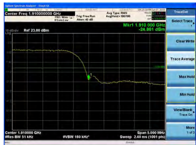
LTE Band 2 1.4MHz QPSK 1RB CH-High
