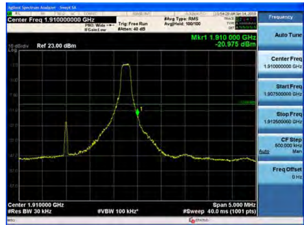
LTE Band 2 3MHz QPSK 100%RB CH-High
