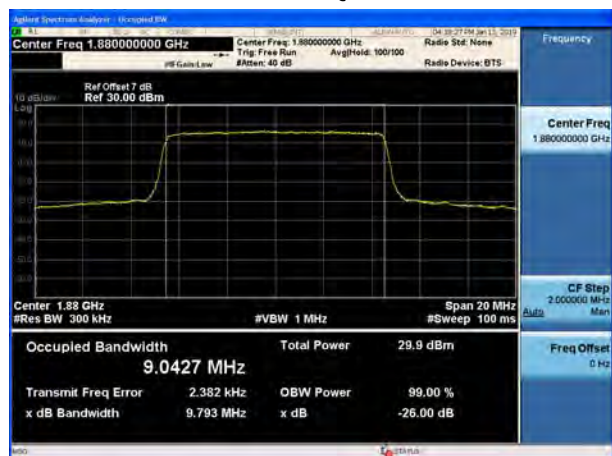
LTE Band 2 10MHz QPSK CH-High
