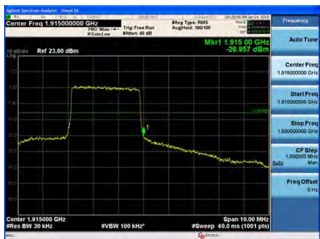
LTE Band 25 5MHz QPSK 1RB CH-High
