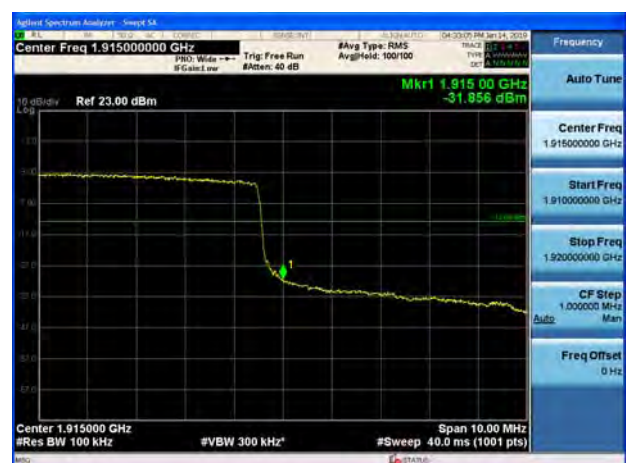
LTE Band 25 10MHz 16QAM 100%RB CH-High
