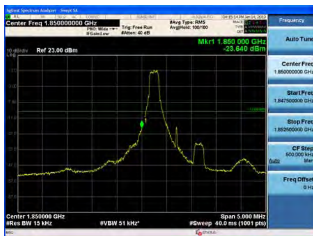
LTE Band 25 1.4MHz QPSK 100%RB CH-Low
