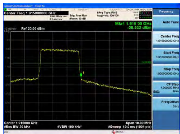
LTE Band 25 5MHz 16QAM 1RB CH-High
