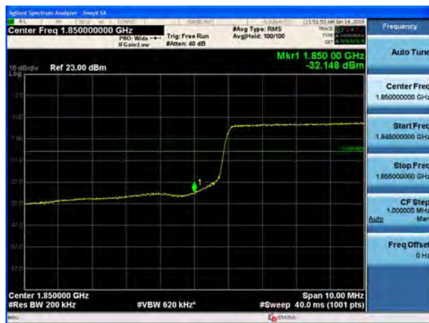
LTE Band 2 1.4MHz 16QAM 1RB CH-Low
