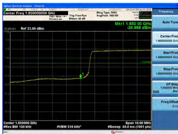
LTE Band 25 20MHz 16QAM 1RB CH-Low
