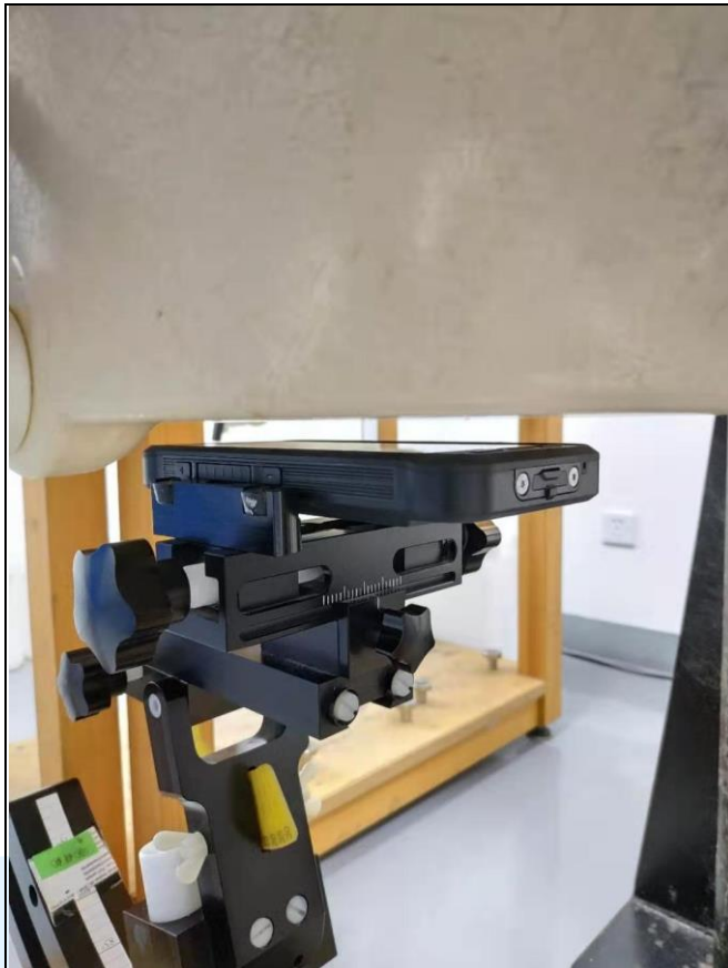
Front Face of EUT with 1.0 cm Gap
