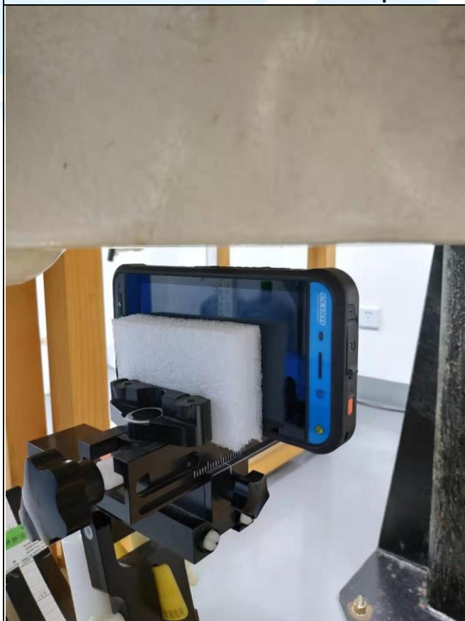
Left Side of EUT with 1.0 cm Gap
