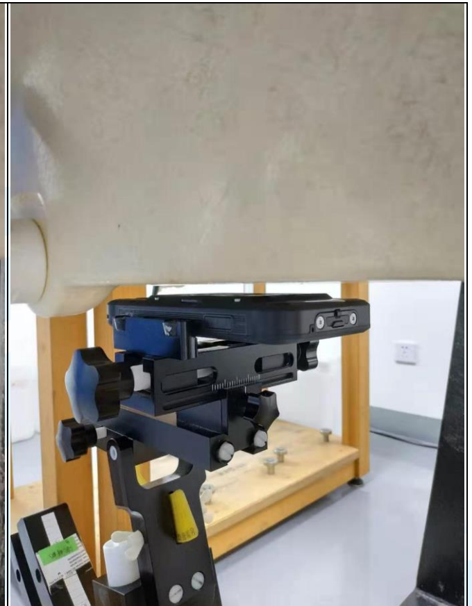
Rear Face of EUT with 1.0 cm Gap
