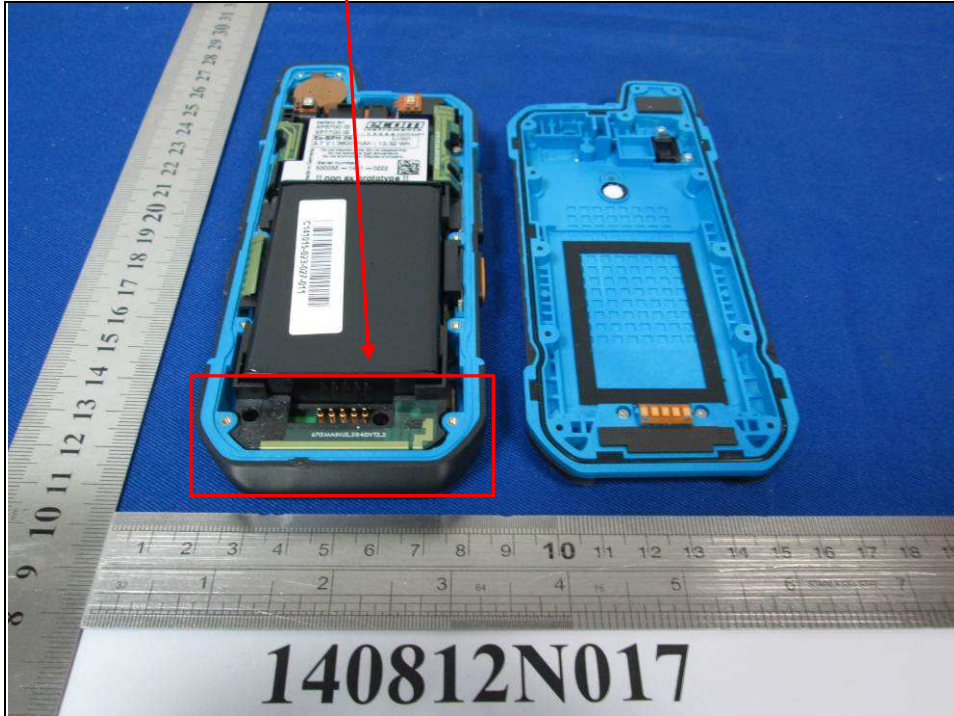
WWAN Main TX/RX Antenna
