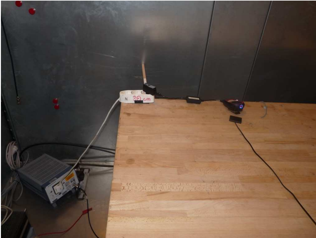
Photo 1: Test setup for conducted measurements on AC port, EUT supplied by AC/DC adapter, used for intentional and unintentional radiator measurements.
