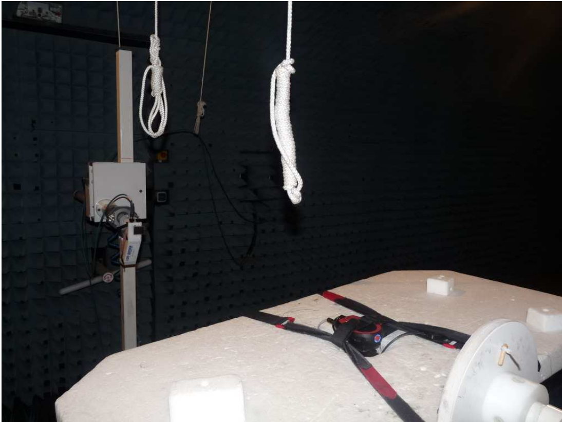
Photo 5: Test setup for radiated measurements in the range 18 – 25 GHz, fully-anechoic chamber, used for intentional radiator measurements.
