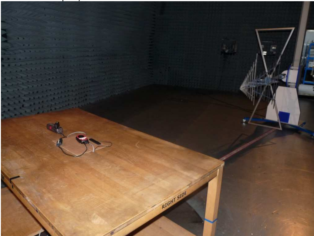
Photo 2: Test setup for radiated measurements in the range 30 – 1000 MHz, EUT supplied by AC/DC adapter, used for unintentional radiator measurements.
