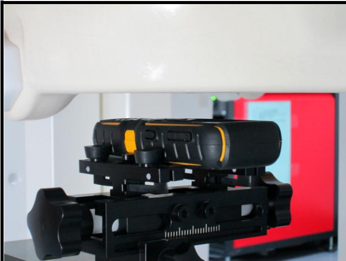
Z1+Battery 1 – Front Face with 1.5 cm Gap
