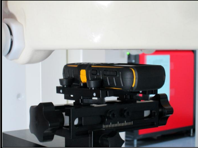
Z1+Battery 2 – Front Face with 1.5 cm Gap
