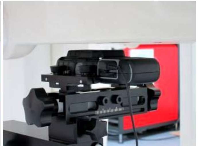
Rear Face of EUT with 1.5 cm Gap
