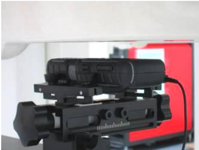
Front Face of EUT with 1.5 cm Gap
