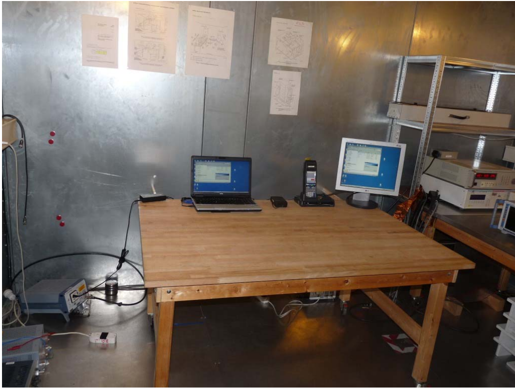
Photo 6: Test setup for conducted measurements (computer peripheral setup, EUT supplied by USB-cable from battery, unintentional radiator §15)
