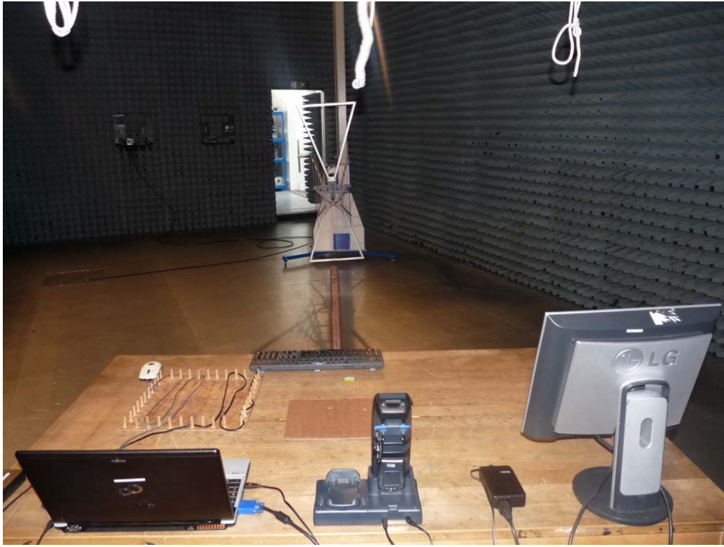
Photo 8: Test setup for radiated measurements (computer peripheral setup, EUT supplied by USB-cable from battery, unintentional radiator §15)
