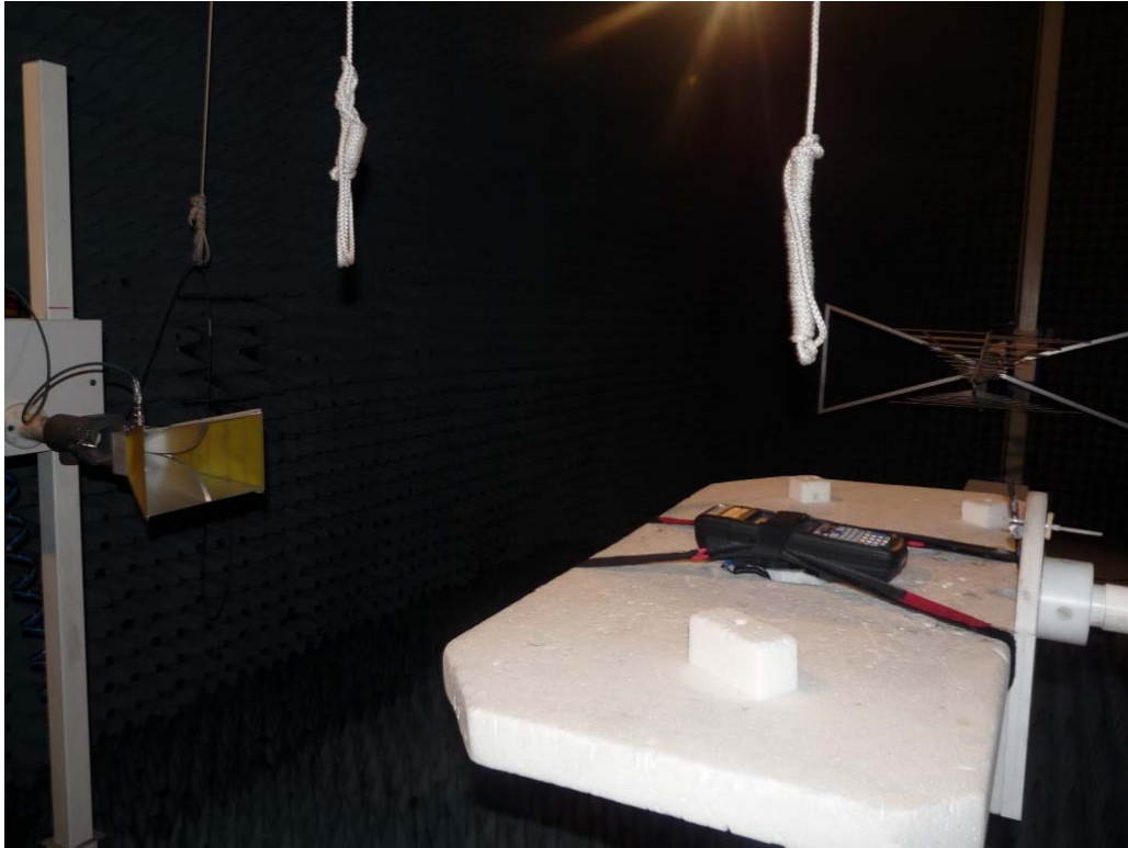
Photo 4: Test setup for radiated measurements (Enclosure, fully-anechoic chamber, 18-25 GHz, intentional radiator § 15)
