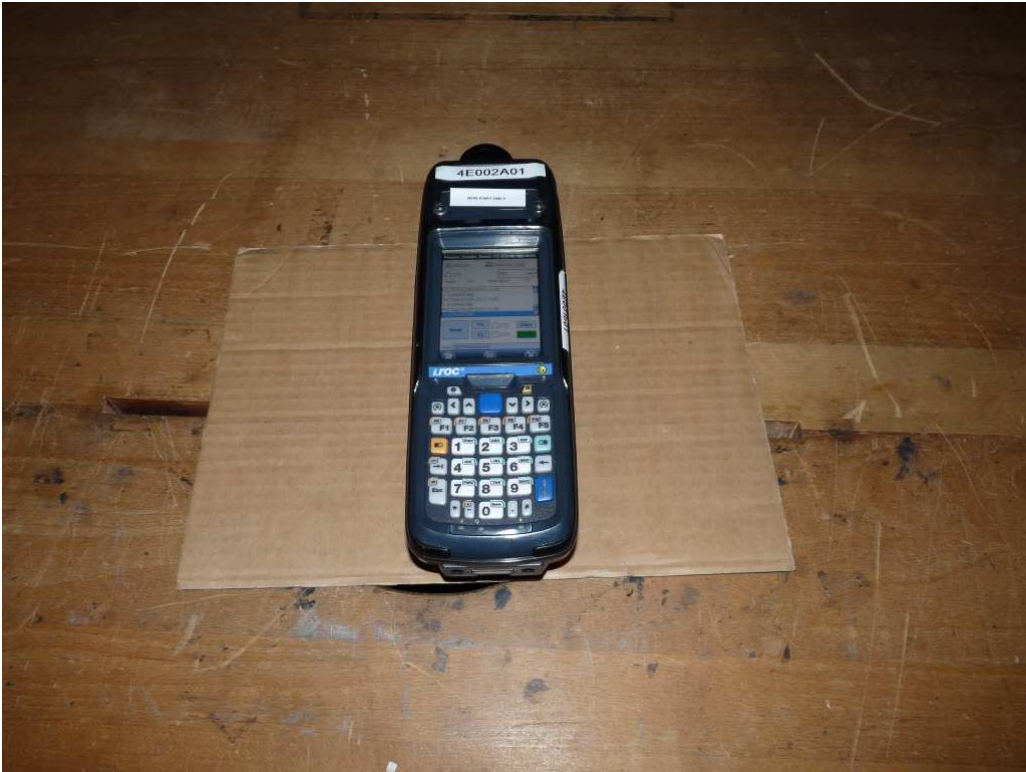
Photo 1: Test setup for radiated measurements (below 30 MHz)
