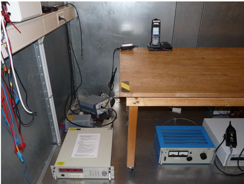
Photo 3: Test setup for conducted measurements
