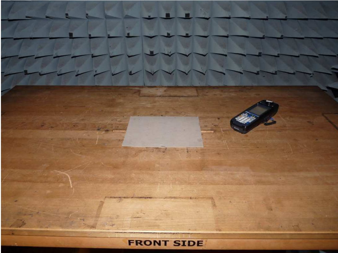
Photo 1: Test setup for radiated measurements (below 30 MHz)
