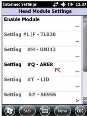
Pic7: Head Module Settings after enabling the ARE Trovan reader
