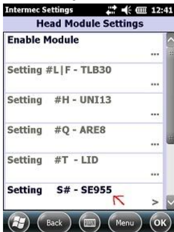
Pic11: Head Module Settings after enabling the SE955 scanner
