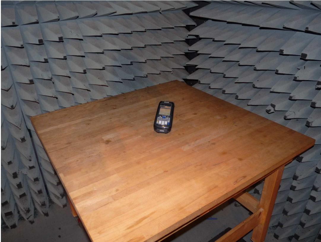
Photo 1: Test setup for radiated measurements (below 30 MHz)
