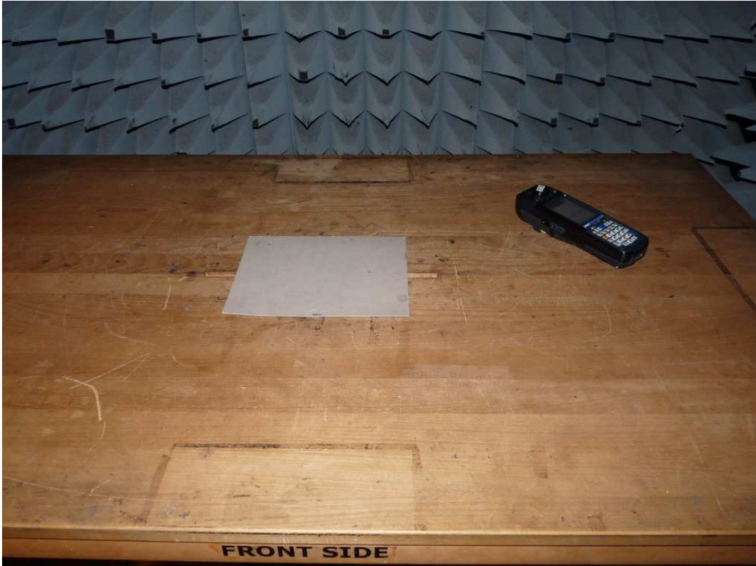
Photo 1: Test setup for radiated measurements (below 30 MHz)
