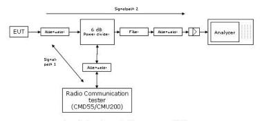
Remark: Depending on the frequency range suitable attenuators and/or filters and/or amplifiers are used.
