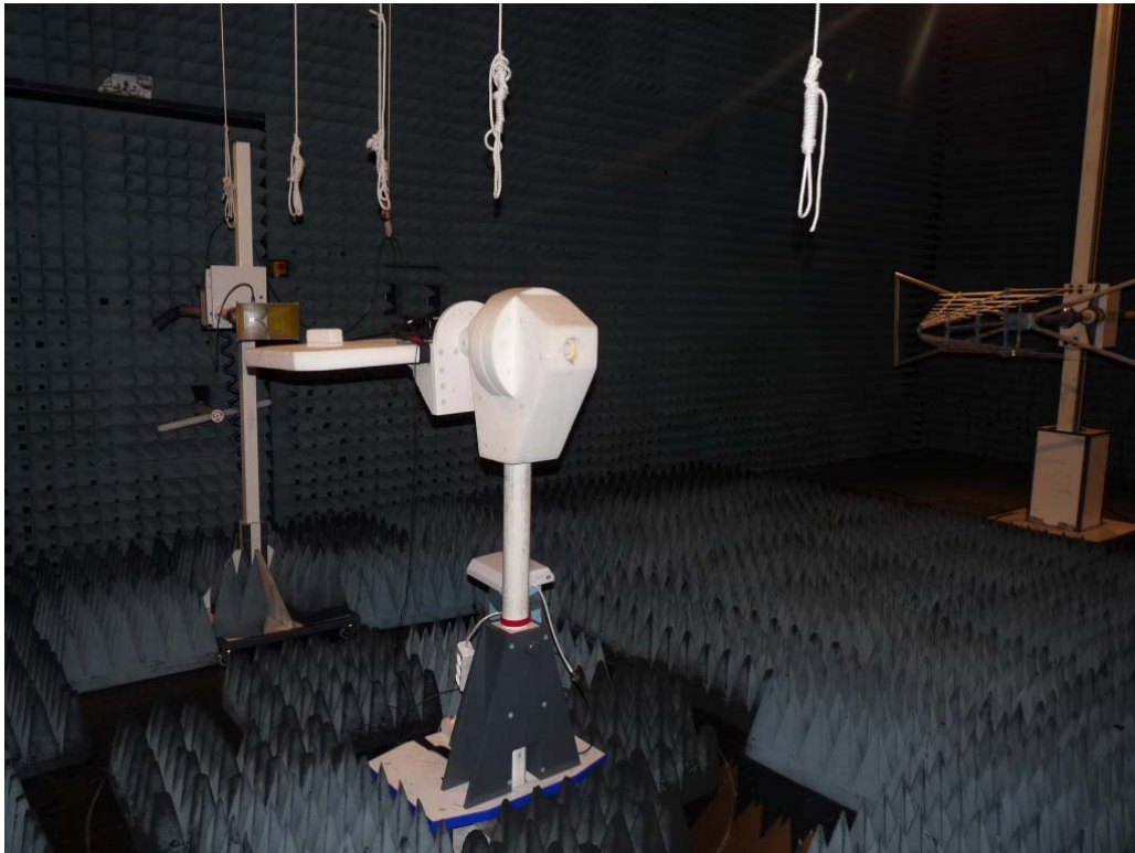
Photo 3: Test setup for radiated measurements (above 1 GHz)
