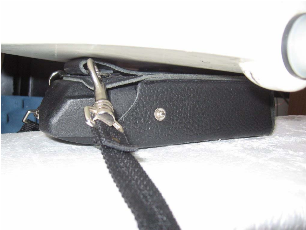
Photo 32: Test position body worn front side (with the 2nd holster) without any distance
