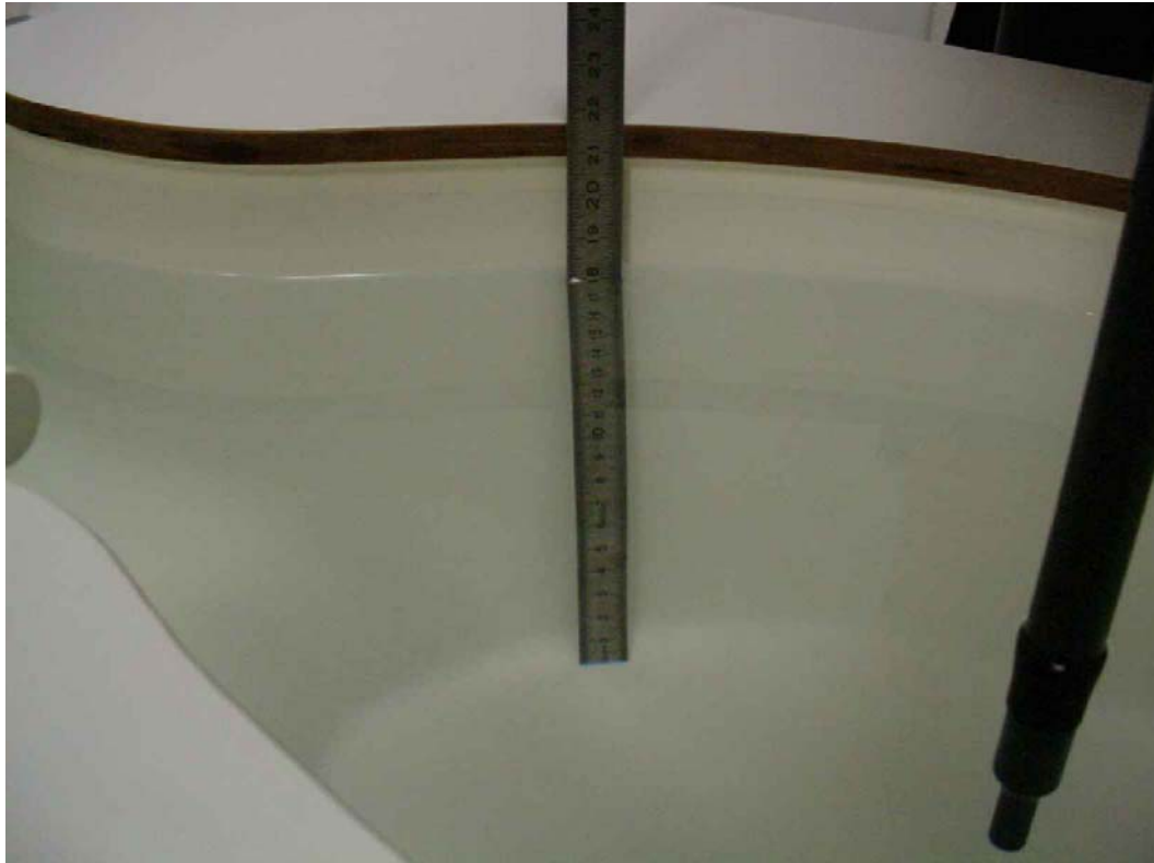
Photo 35: Liquid depth 2450 MHz body simulating liquid
