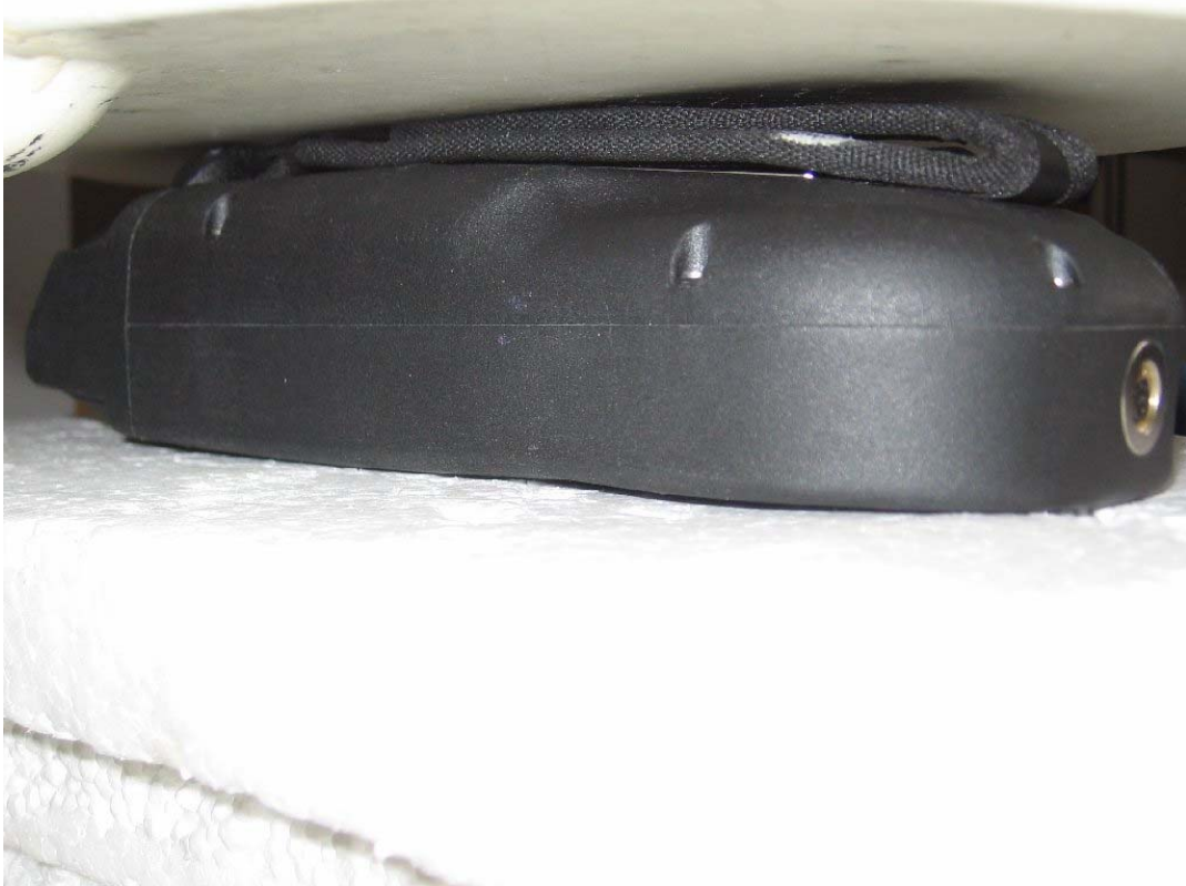
Photo 28: Test position body worn front side (with the 1st holster) without any distance
