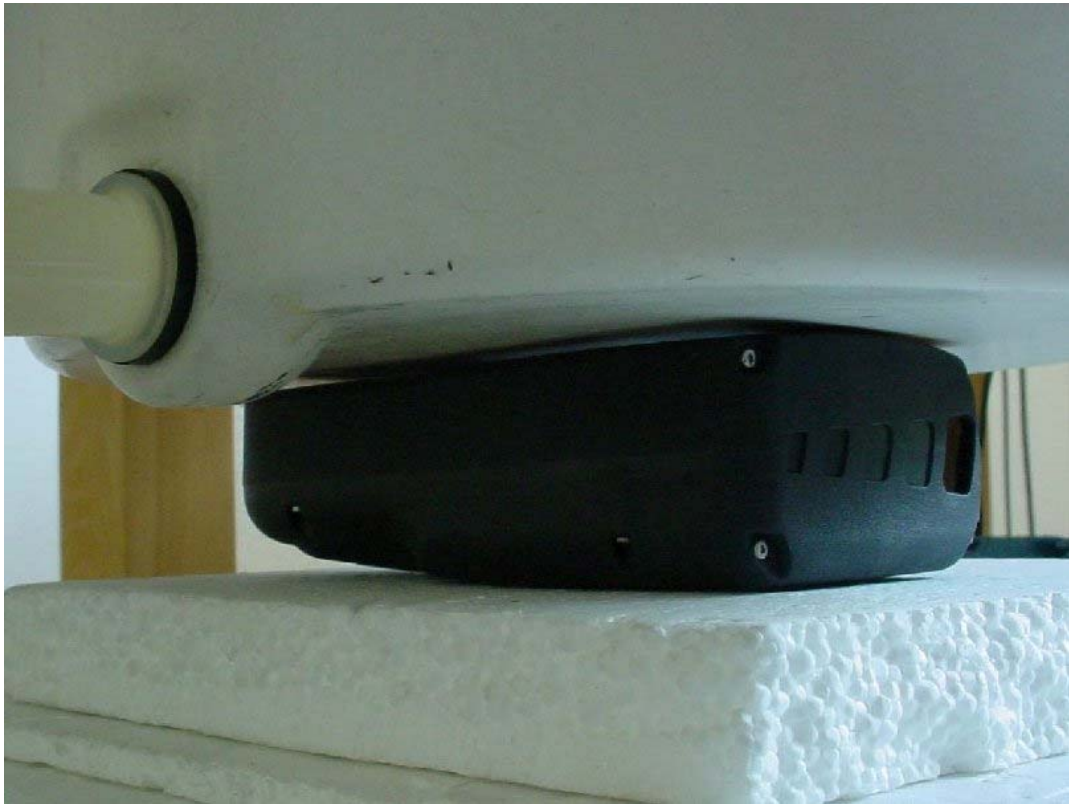
Photo 34: Test position body worn rear side (without RFID-Module) without any distance
