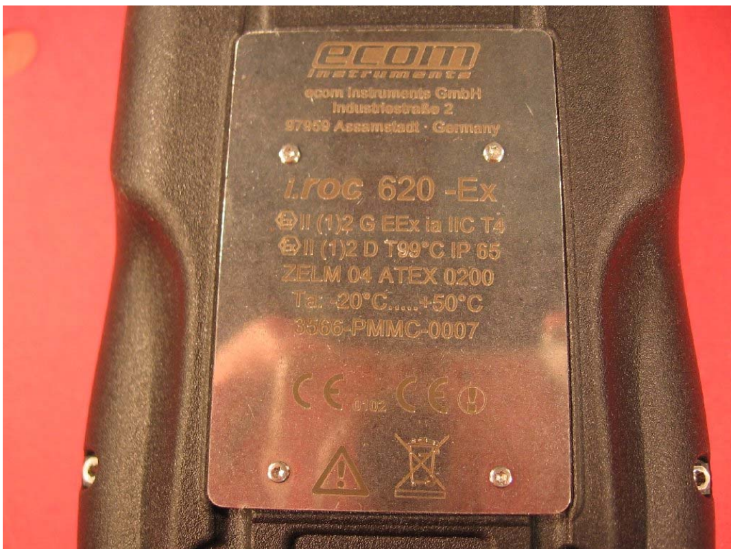
Photo 8: DUT #2 - rear view (label)
