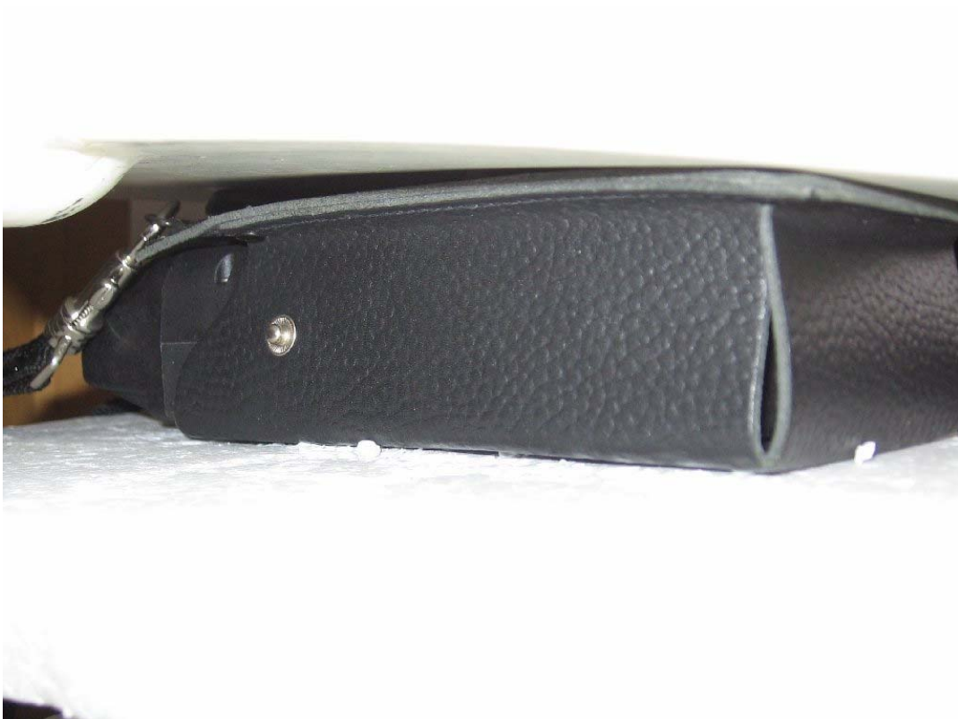
Photo 30: Test position body worn rear side (with the 2nd holster) without any distance
