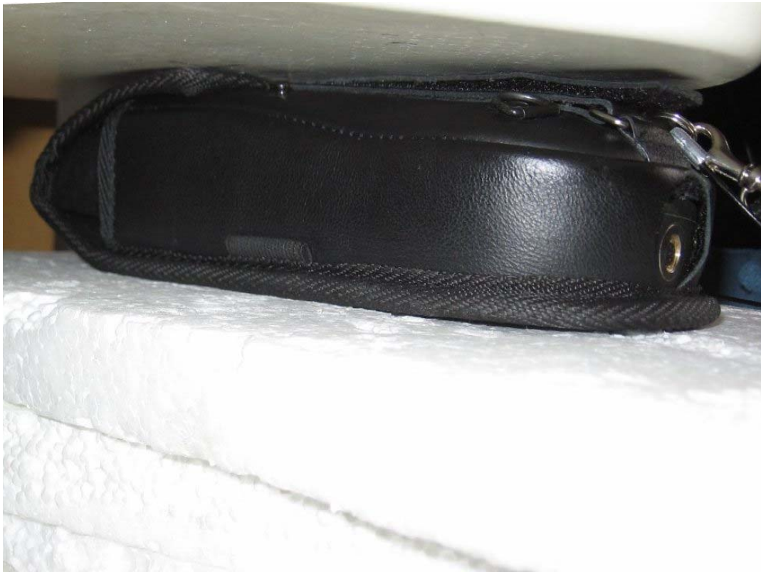
Photo 30: Test position body worn rear side (with the 2nd holster) without any distance
