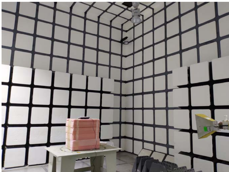
Radiated Emissions View (Above 1 GHz)
