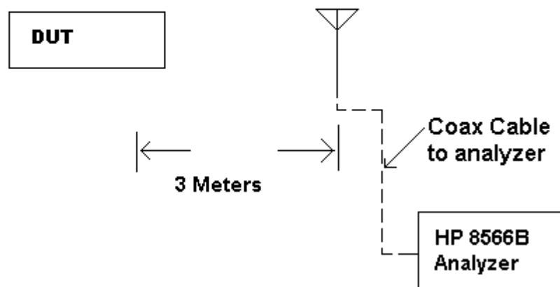
**METHOD OF MEASUREMENT:** The procedure used was ANSI standard C63.4-2003 & the FCC/OET Guidance on Measurements for Spread Spectrum Systems – Public Notice DA 00-705 dated March 30<sup>th</sup>, 2000.
