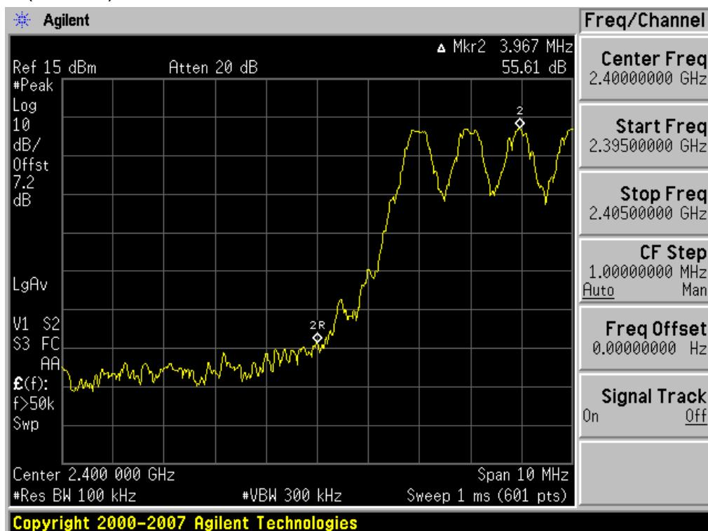
Test Plots with hopping (GFSK)
