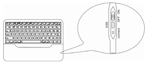
(2). While the battery is charging the connect light in red will illuminate. When charging is completed the light will turn off. Charging time is 2.5 hours
