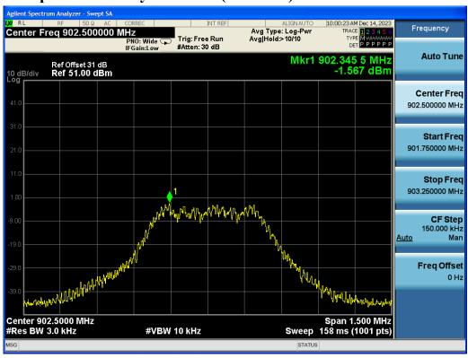
**Power Spectral Density Test Plot (CH-Mid)**
