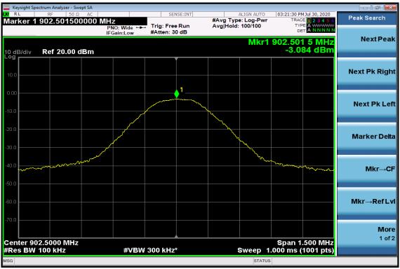
**Power Spectral Density Test Plot (CH-Mid)**
