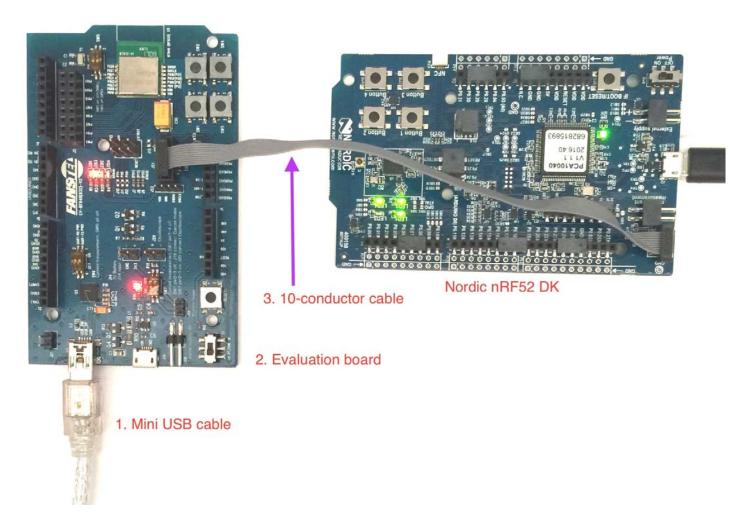
• 10-conductor cable for connection to Nordic nRF52 DK (DK is not included)
