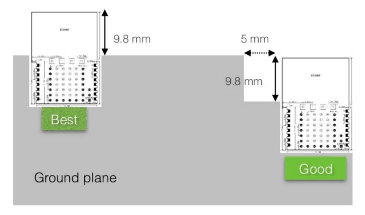
• We don't recommend mounting BT840X module in the middle of a host PCB.
