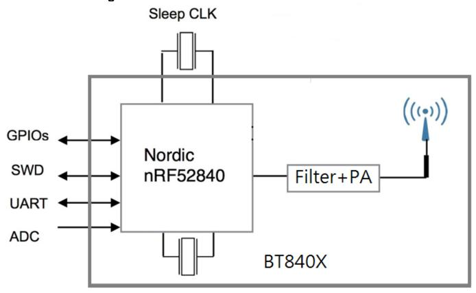
BlurNor BT840X is a sister module of BT832F. The physical size is the same. There are 21 additional LGA pins for additional GPIOs provided by nRF52840.
