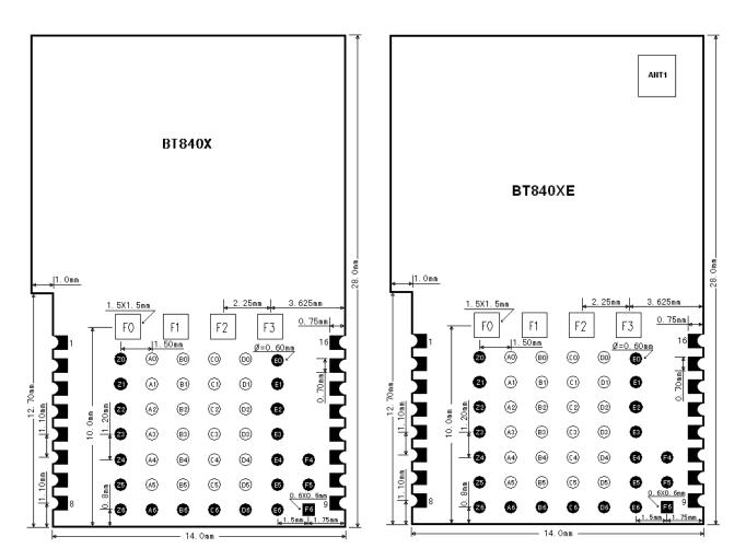
BT840X and BT840XE mechanical drawings
