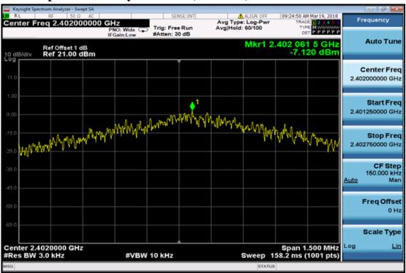
**Power Spectral Density Test Plot (CH-Mid)**
