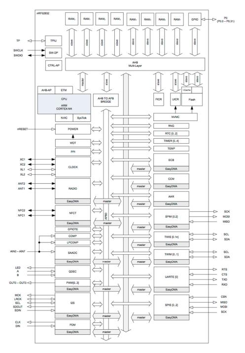
The following is a block diagram of Nordic nRF52832 SoC.
