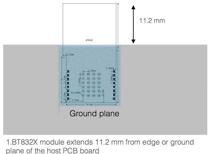
2.Except required for pin connection, ground plane on top layer of main board.
