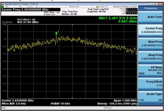
**Power Spectral Density Test Plot (CH-Mid)**
