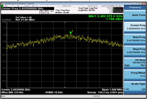
**Power Spectral Density Test Plot (CH-Mid)**
