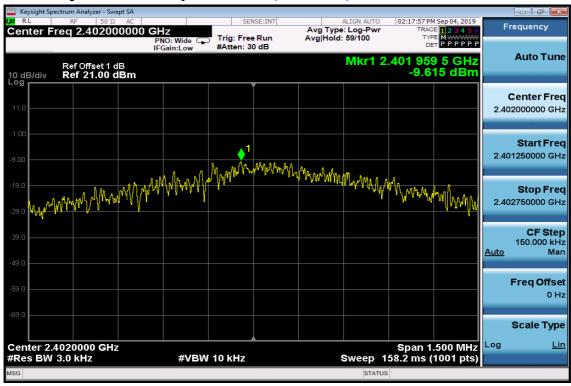
**Power Spectral Density Test Plot (CH-Mid)**
