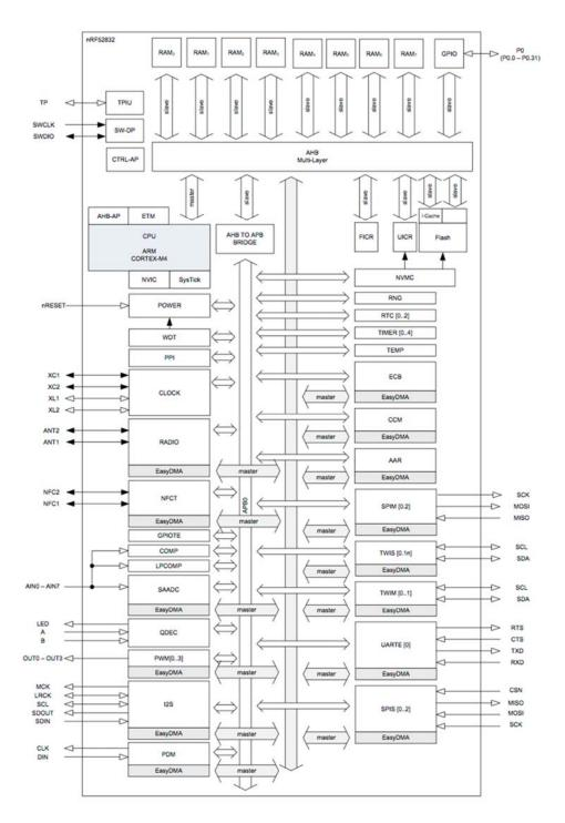
The following is a block diagram of Nordic nRF52832 Bluetooth Low Energy (BLE) SoC. NFC is not supported .
