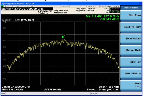
**Power Spectral Density Test Plot (CH-Mid)**
