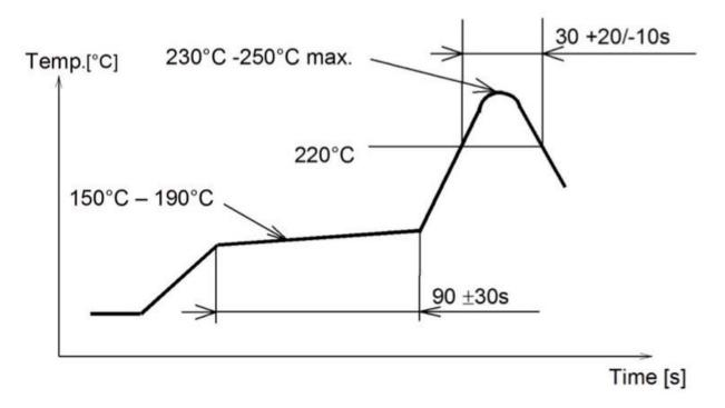
The following temperature profile is suggested for re-flow oven.
