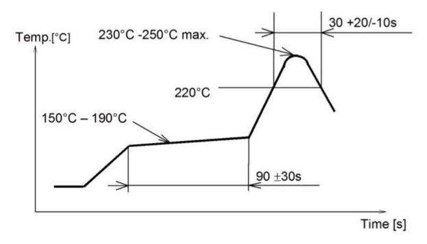
Maximum number of cycles for re-flow is 2. No opposite side re-flow is allowed due to module weight.
