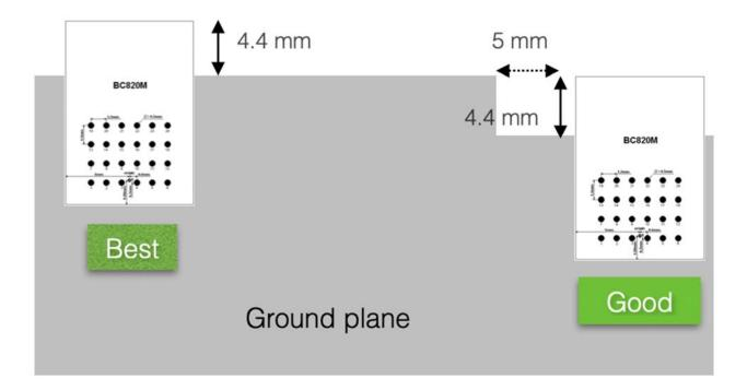
• We don't recommend mounting BC805M module in the middle of a host PCB.
