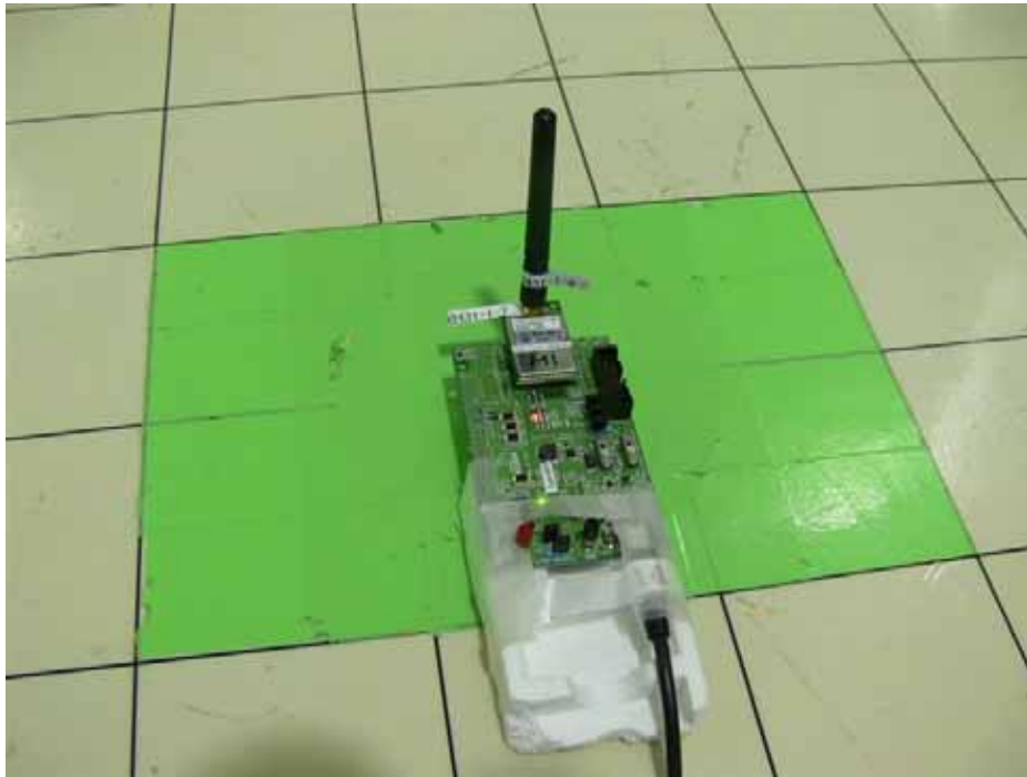
Photograph 10: Set-up for Radiated Emission, EUT Configuration X-Axis
