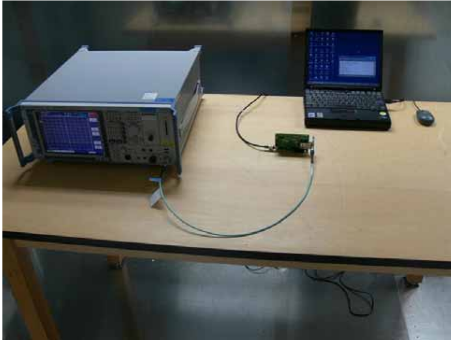
Photograph 1: Set-up for Conducted Emissions at Antenna Port
