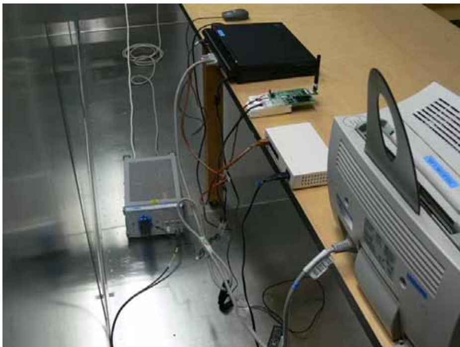
Photograph 5: Set-up for AC Power Line Conducted Emission of Receiver, Rear View
