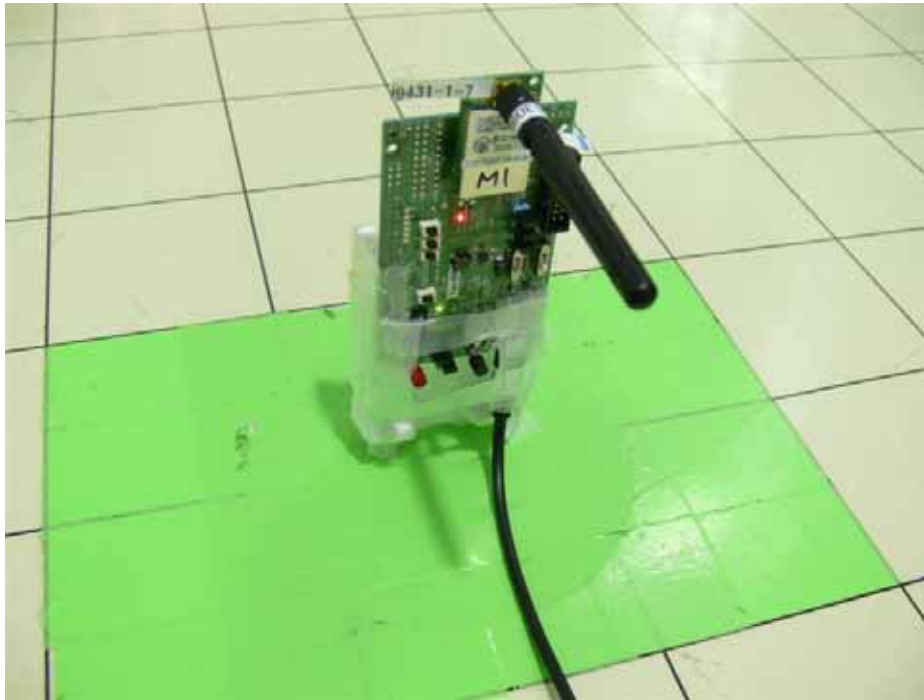
Photograph 12: Set-up for Radiated Emission, EUT Configuration Z-Axis
