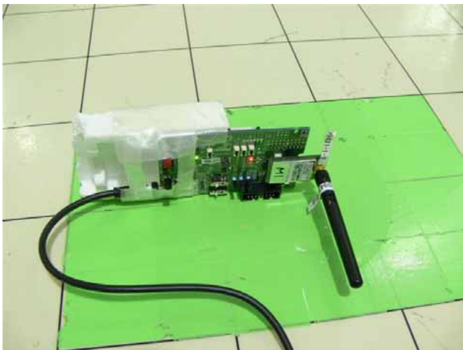
Photograph 11: Set-up for Radiated Emission, EUT Configuration Y-Axis
