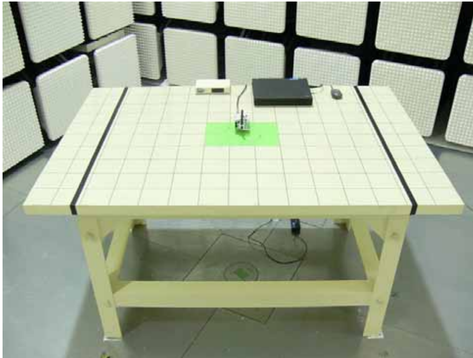
Photograph 6: Set-up for Radiated Emission of Transmitter, Front View
