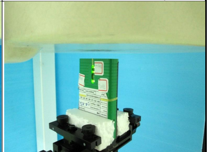
Bottom Side of EUT with 1.0 cm Gap
